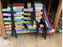
Cutting wood precisely to size, drilling holes, and finishing wood pieces is all done in Auburn or Woodinville then sent to Spokane, where it is hooked for painting, primed, and colorfully painted (l-r) ready to be hooked; painted and drying; seats ready for assembly.
